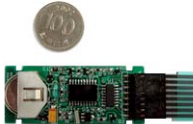
Slim controller with coin cell battery (1~6 weeks lifetime)
