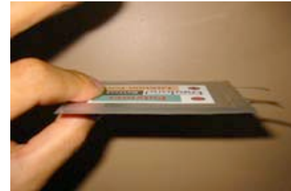
Slim controller with rechargeable battery (2~4 months lifetime)
